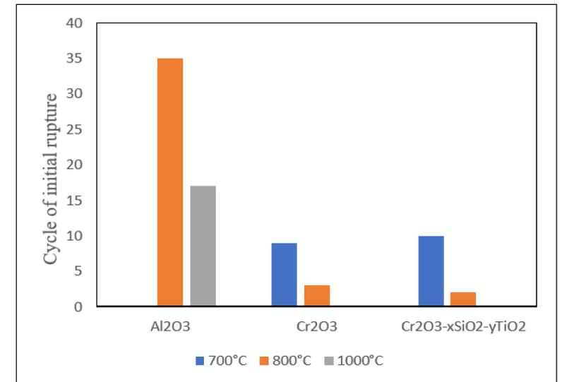
Figure 2. Results of thermal shock tests
